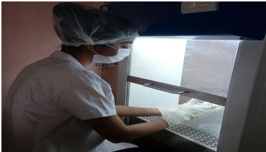
Plate 4. Serial dilution and Plating done under Laminar Air Flow
